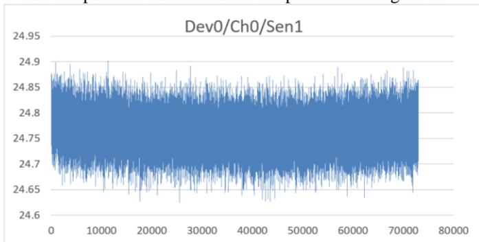
Fig. 5 Temperature FBG sensor measurement graph. Where the X-axis represents the number of samples and Y-axis the temperature in degrees Celsius.
