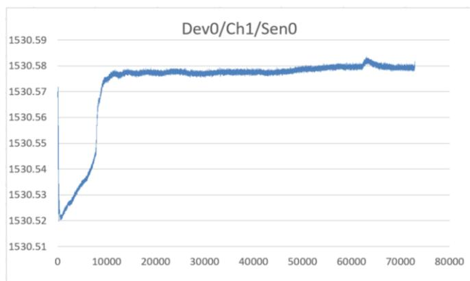
Fig. 8 RH FBG sensor measurement graph. Where the X-axis represents the number of samples and Y-axis the wavelength in nm.
