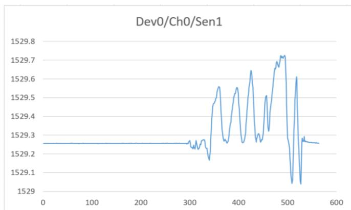
Fig. 7 Strain FBG sensor measurement graph. Where the X-axis represents the number of samples and Y-axis the wavelength in nm.
