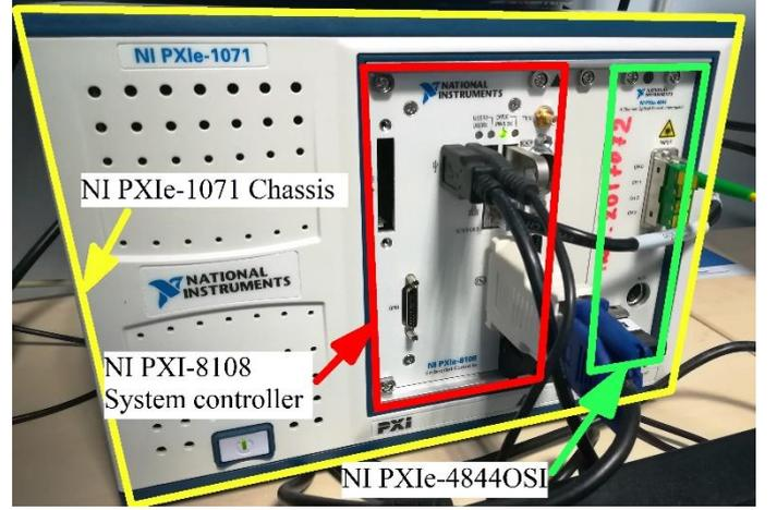
Fig. 3 Data acquisition hardware.
