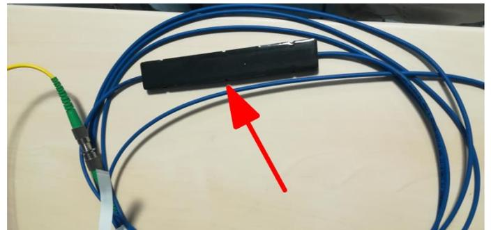
Fig. 6 Strain FBG sensor.
