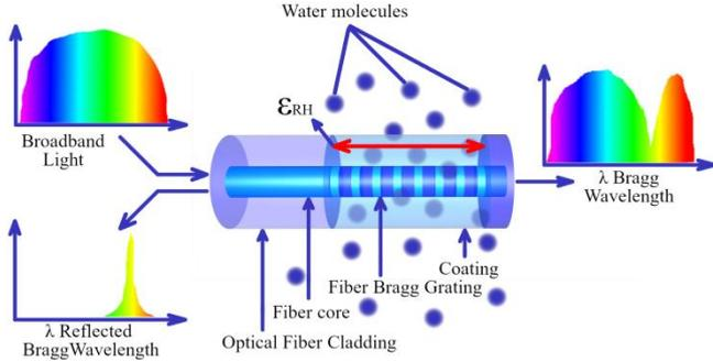
Fig. 2 RH FBG coated sensors.
