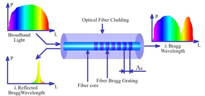
Fig. 1 Basic FBG sensor functionality.
