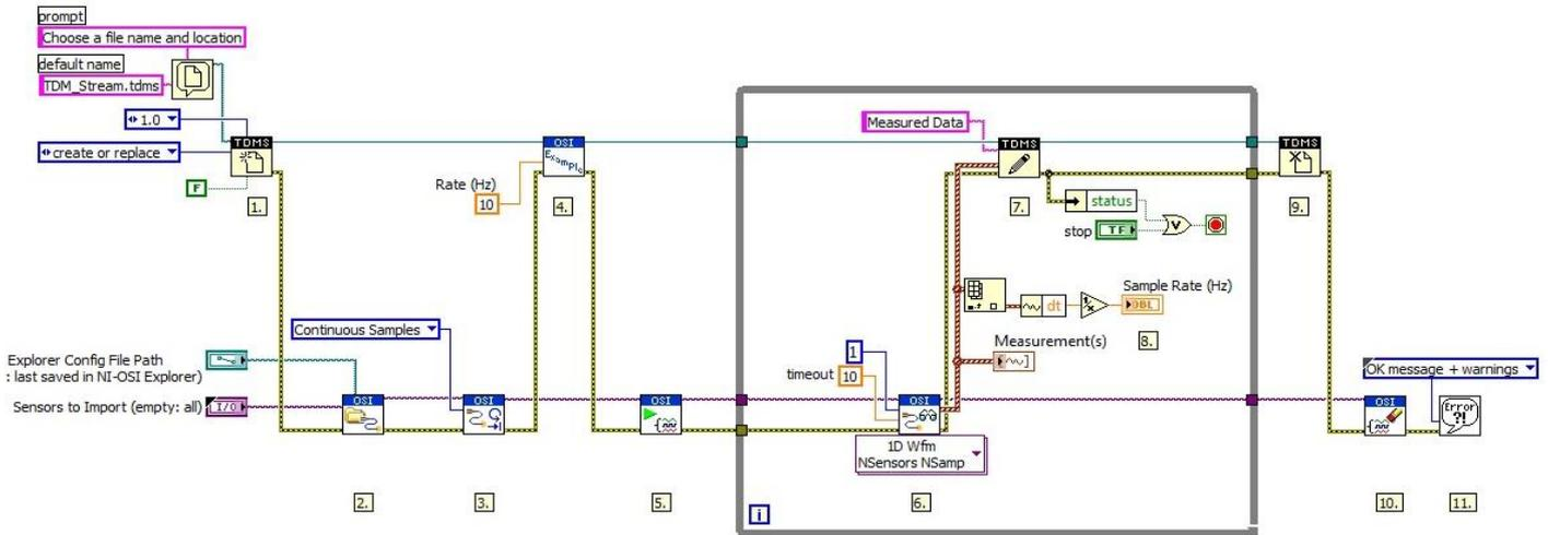
Fig. 4 LabVIEW Block Diagram of the data acquisition system.
